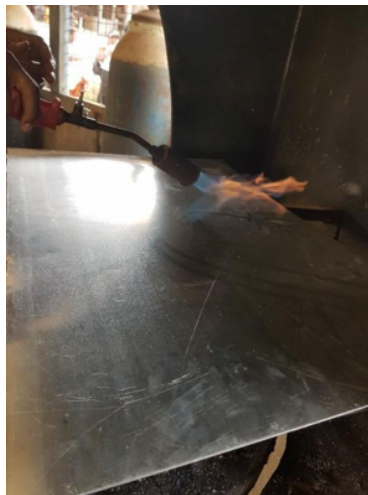
Figure 4. Annealing the aluminium sheet (July 2021).
