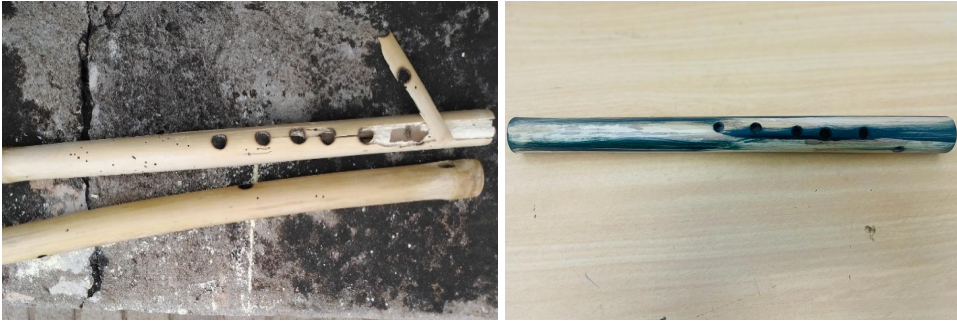
Figure 10: on the left is an atenteben with insect attack and right is another atenteben with wood dent. Photograph by researcher.
