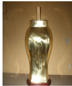
Figure 11: Lampshade-Stand after it was Polished with Bar Polishing Compound.
