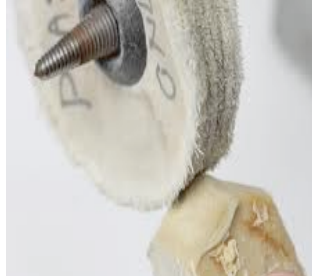
Figure 7: Impregnating the Polishing Wheel with Polishing Compounds.
