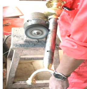
Figure 8: Polishing with Motor Secured on a Bench in Metal Design Studio.
