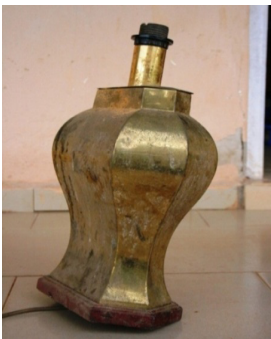
Figure 9: The Surface of a Brass Lampshade-Stand before Polishing Operations is Applied.
