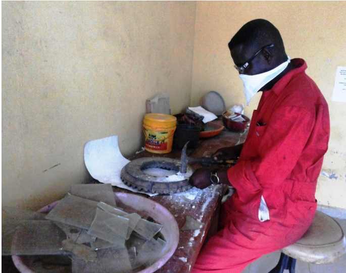
Figure 16: Crushing Broken Glass Using Hammer and Cast Steel Metal.
