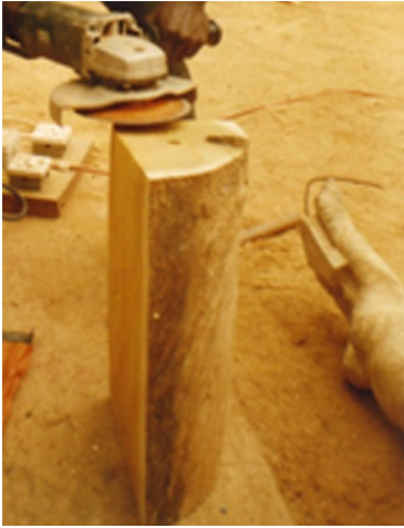
Plate 10. Grinding with Sanding Device.
