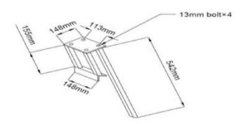
Fig 1 Seat for the motor
