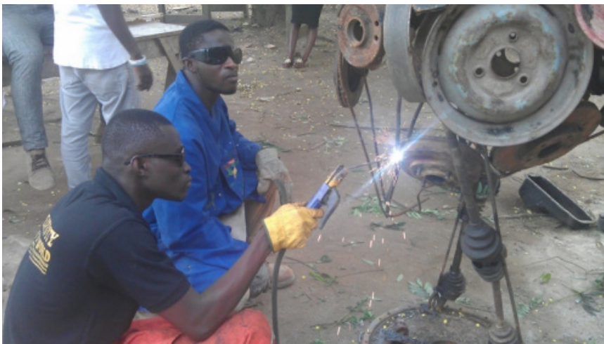
Figure 11 (B): Arc welding processes of scrap metals into composition
